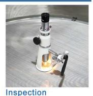
Before the vibrating screen is shipped, we use a microscope and a tension tester to check that the specifications of the vibrating screen mesh comply with the contract requirements and standard.
